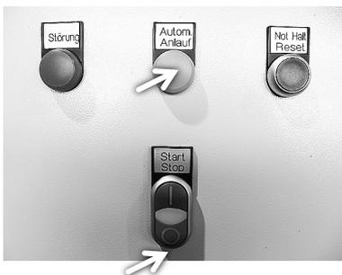
During **Automatic operation**, the motor of the connected macerator starts according to the signals of the pump control unit<sup>1)</sup>.
