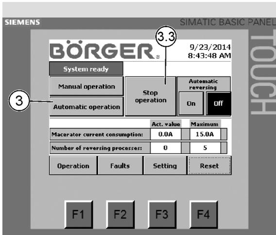
**3 Automatic operation:** Operating mode, to be activated for controlled operation according to the pump control unit, flashes alternatingly in light and dark gray when activated
