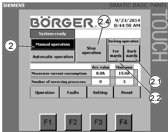
2 **Manual operation:** Operating mode, to be activated for unregulated operation as well as for inching operation (e.g. for manual reversing), highlighted in dark gray when activated
