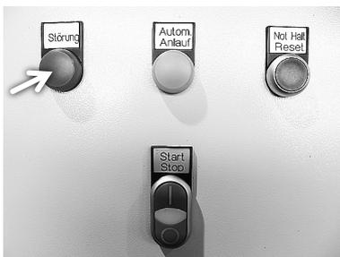
If the current consumption of the macerator motor still exceeds the preset limit after completing the **Maximum** number of automatic reversing processes within ten minutes, the control unit switches off the motor of the macerator. The red LED indicator lamp **Fault** lights up.
