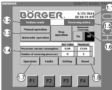
If the current consumption of the motor of the connected macerator exceeds the preset limit, the reversing process is initiated.
